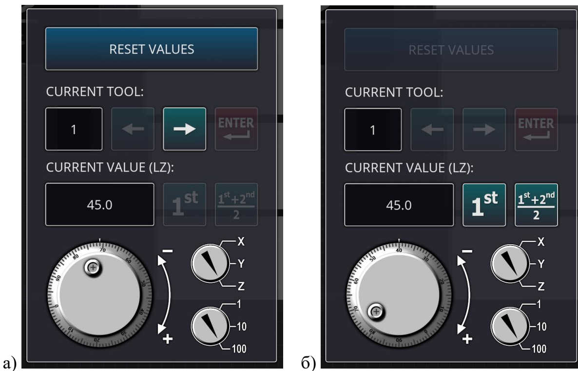
Figure 17 – View of the control panel for the tool binding process in positioning mode (a) and in the measured value recording mode (b)
